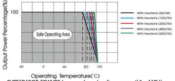
SURF1D12QB-50WHR3 temperature derating curve (Vin=110V)
